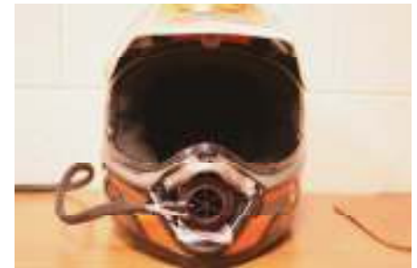
Modified Helmet for VO 2 testing
